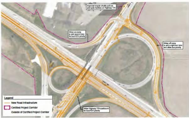
Figure 3: Highway 17A-Highway 99 Interchange Improvements
