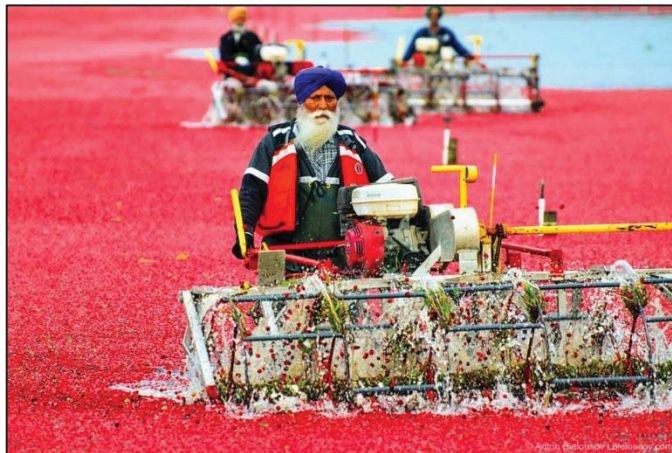
PHOTO 8. CRANBERRY THRESHING MACHINE DURING WET PICK IN OCTOBER. Photo Credit: Anton Bielousov. http://sakvoiazh.ru/
