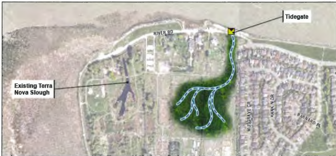
Figure 3: Option 4: Conceptual Diagram of the Alternative Intertidal Marsh Slough in the Northeast Corner of Terra Nova
