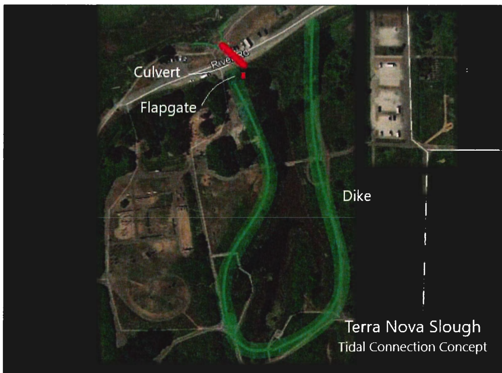
Figure 6: Option 2 – Open Culvert and Ring Dike
