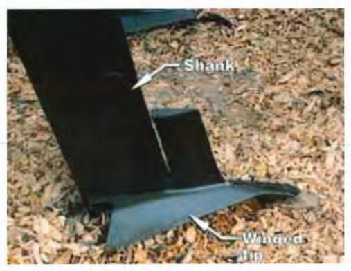
Figure 11 Example of a winged tine subsoiler
