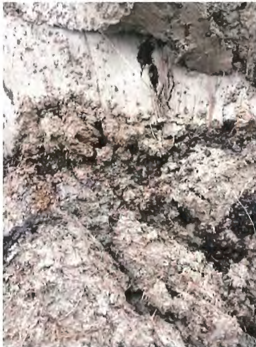
PHOTO 7: SILT LOAM (LESS COMMONLY, SILTY CLAY LOAM) FOUND IN THE CG HORIZON. NOTE DECOMPOSED PLANT MATERIAL PRESENT IN THIS SAMPLE.
