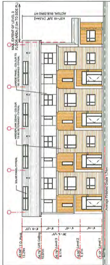
SOUTH ELEVATION (STREET) - BUILDING 2 SCALE: 1/8" = 1'-0"
