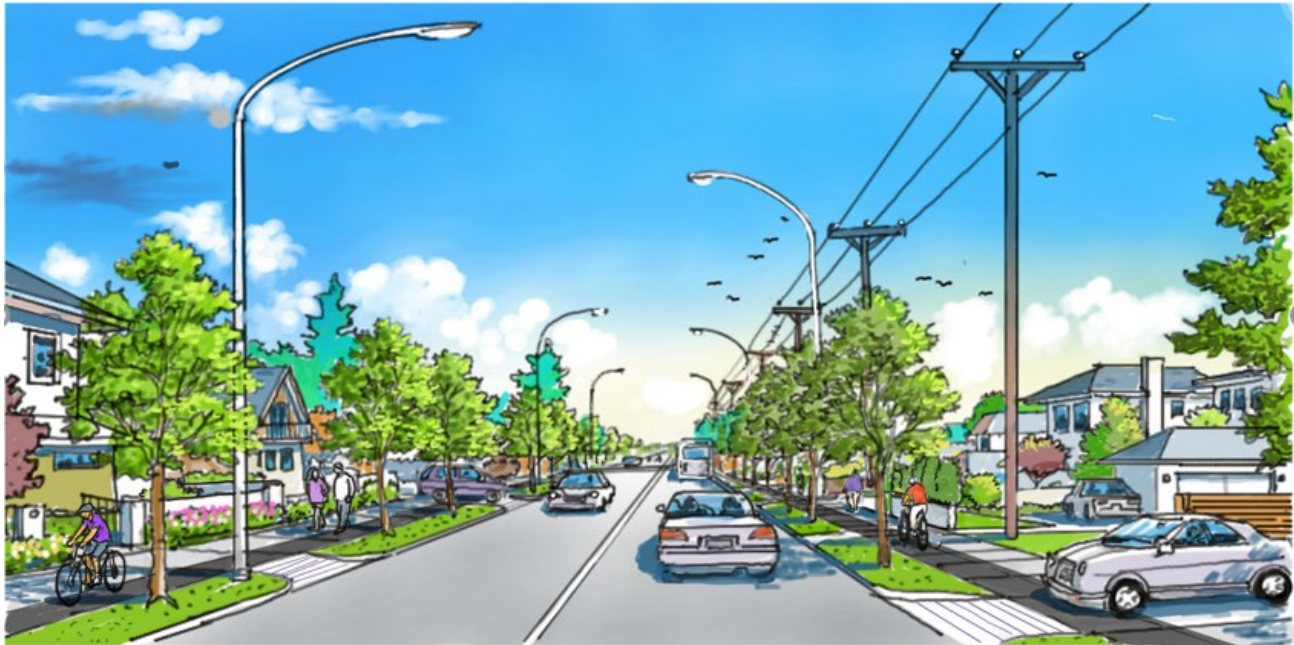
Figure 5: Williams Road Protected Bike Lanes Concept: Typical Cross Section
