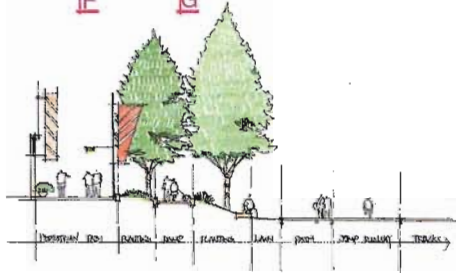
Section B through berms and ramp
