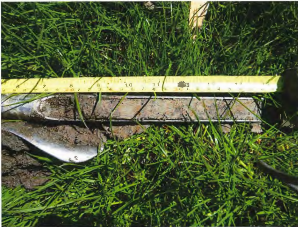
Figure 3 Soil sample showing mottled Bg horizon
