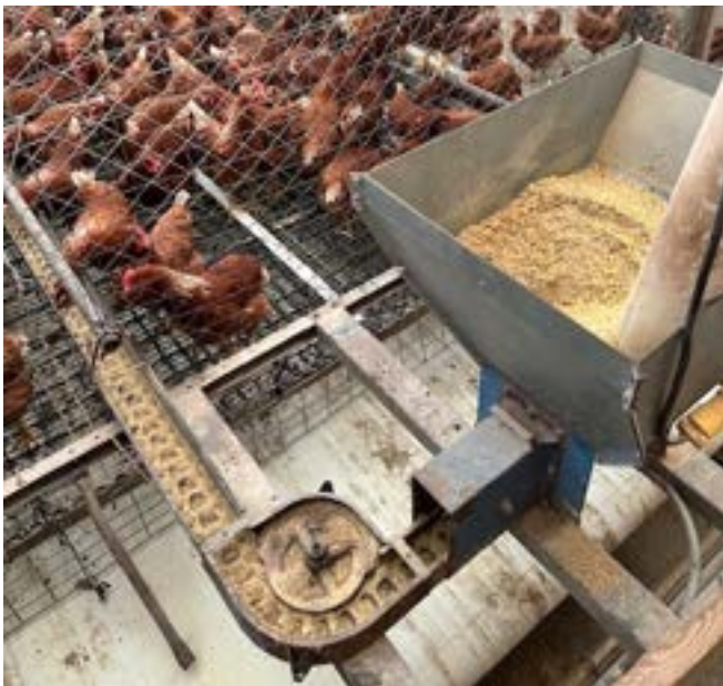
(c) Feed hopper and feed conveyor mechanism.
