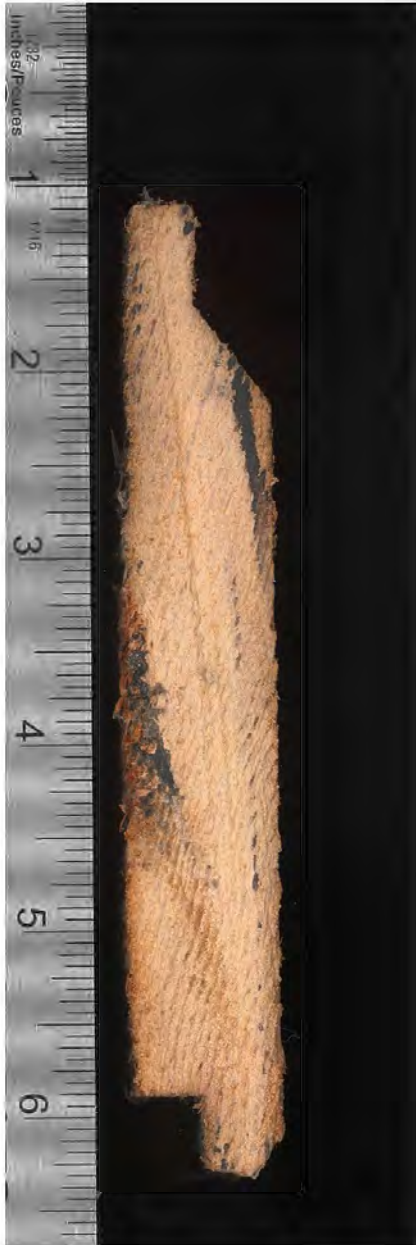
Left: profile of original 1894 Fir drop siding.
