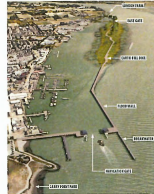
▲ FIGURE: A look from above at what the Steveston Island Dike could look like when built.
