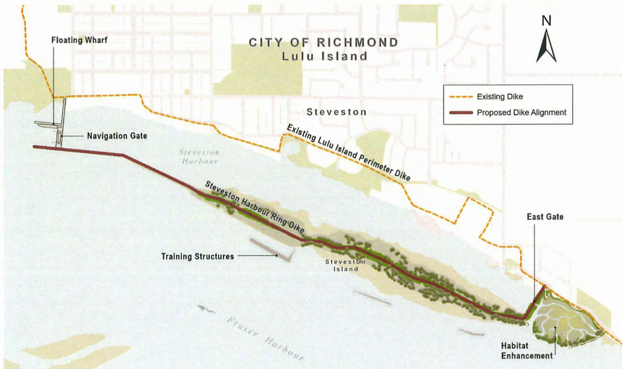
Figure 1: Steveston Island Dike Layout
