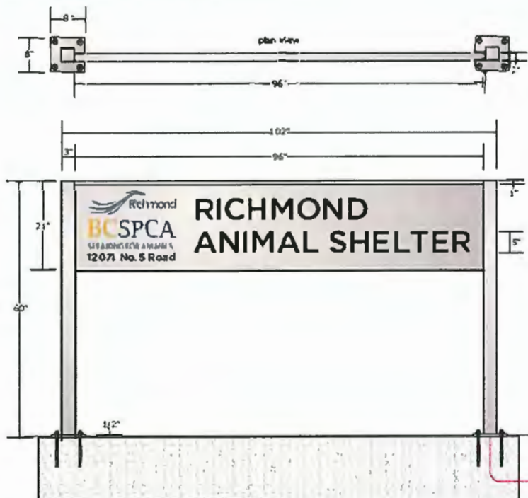
Figure 5. Building signage at entrance to RAS driveway. Overall dimensions 5' high x 8' 6" length
