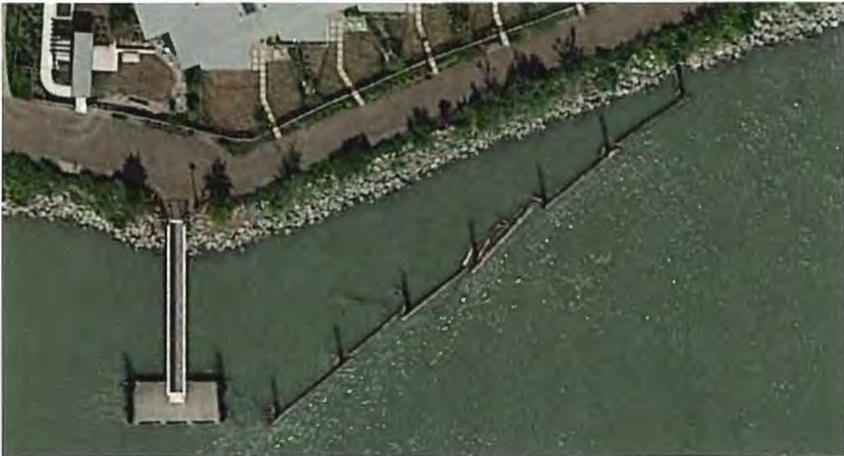
Figure 1 Debris deflection boom at Queensborough (source: GoogleEarth).
