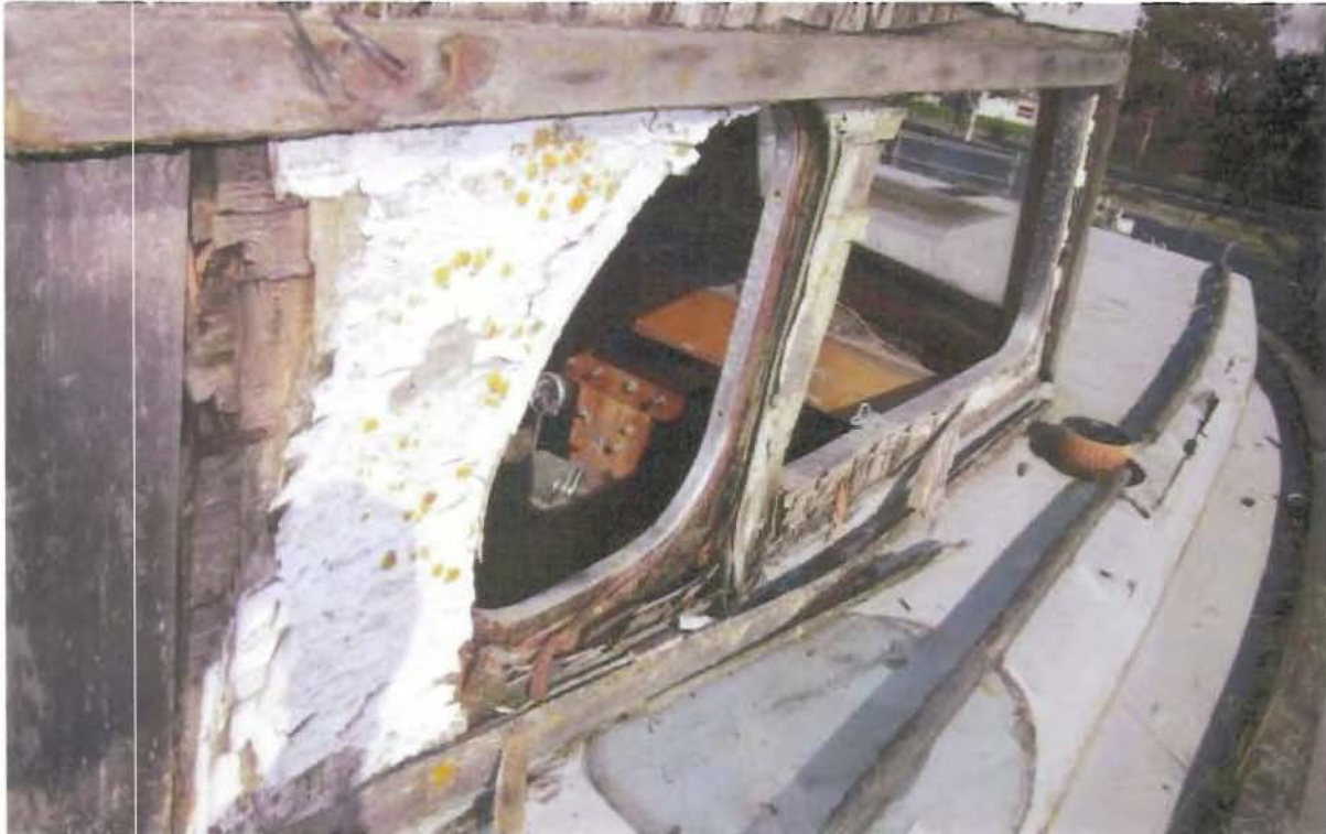
Photo # 3 Heavily deteriorated superstructure
