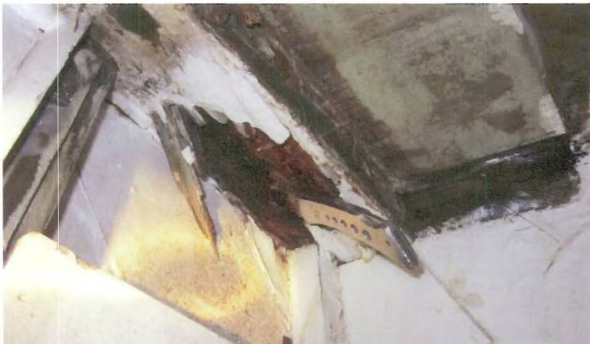
Photo #5 Deterioration of sheer clamp forward cabin
