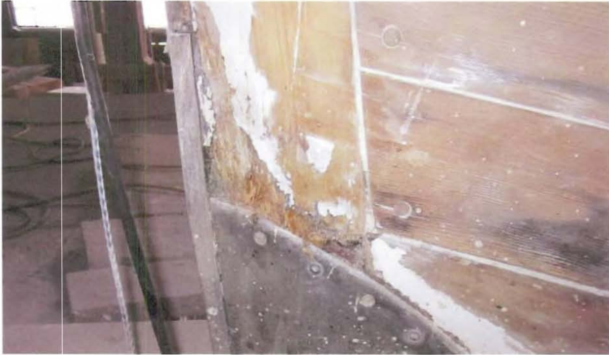
Photo #1 Damage of exterior stem structure
