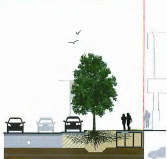
"ENGINEERED" | OPEN VOLUME + STRUCTURAL / CONSTRUCTED SOIL VOLUME
