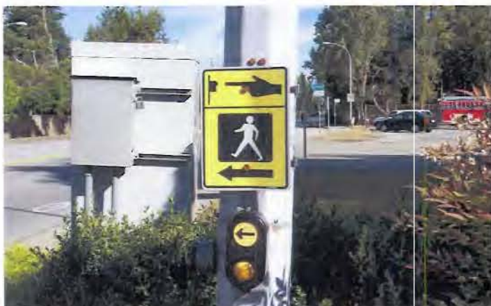
New enhanced accessible pedestrian signal devices will help people living with disabilities safely cross roadways.
