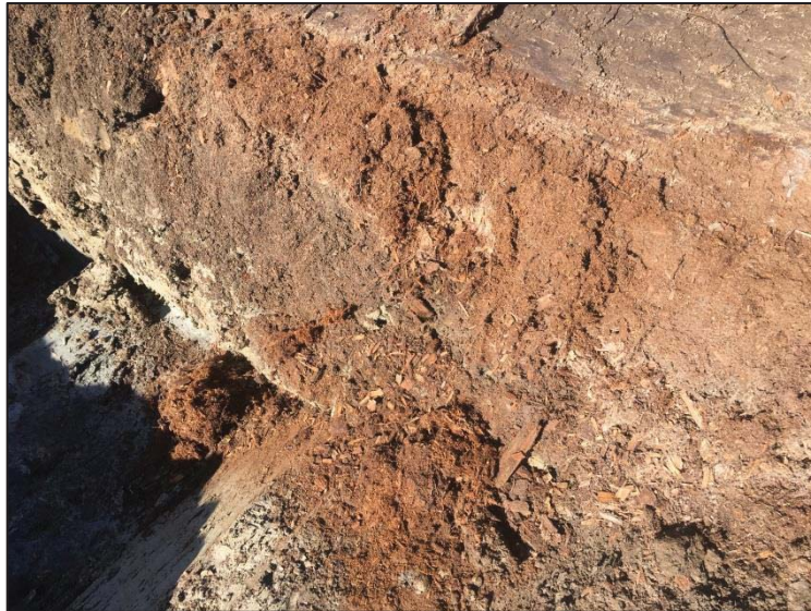
PHOTO 3. WOOD SHAVINGS PRESENT AT THE TOP OF THE AH LAYER IN SOIL PIT 7.
