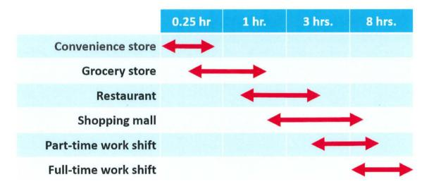
The scenarios in the table above indicate that the delivered charging capacity for rapid-turnover parking spaces should be higher than that provided to stalls where vehicles will be parked for several hours or longer.
