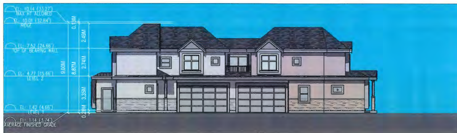
4 BUILDING B WEST ELEVATION SCALE: 1/8"=1'-0"
