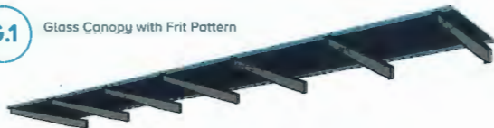
Glass canopy with exposed outriggers.
