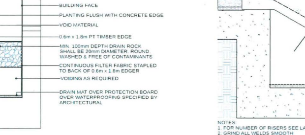
7 GRAVEL DRAIN STRIP - ON SLAB Scale: 1:10
