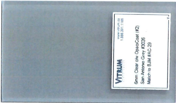
RESID'L TOWER SPANDREL PANEL COLOUR 1 BM-AC-29
