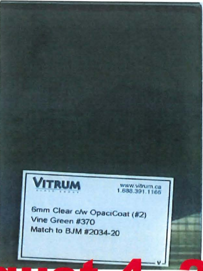
RESID'L TOWER SPANDREL PANEL - COLOUR 2 BM-2034-20
