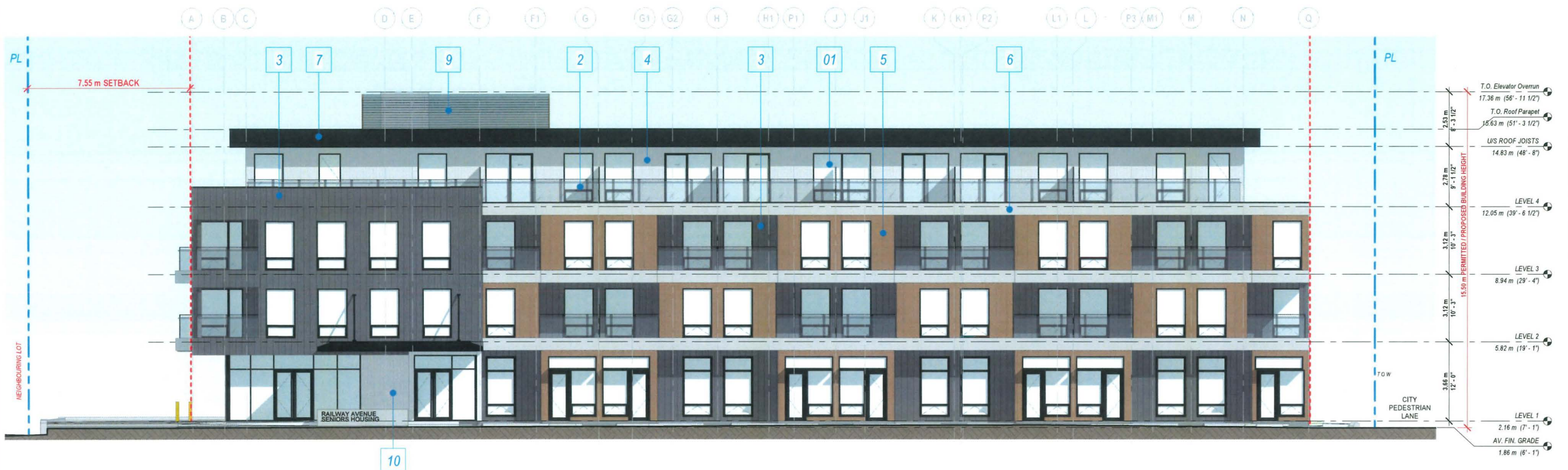
1 WEST ELEVATION - ALONG RAILWAY AVENUE SCALE: 1/8" = 1'-0"
