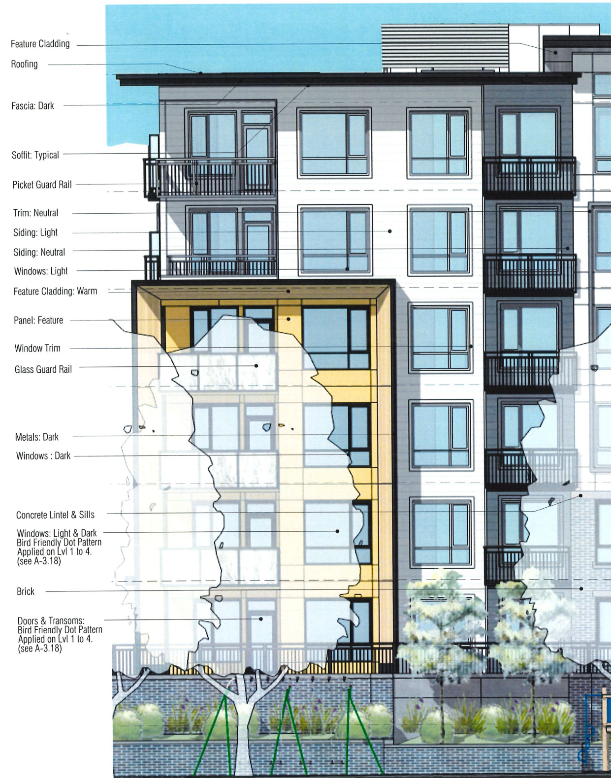
Roofing 2-Ply SBS Roofing Coloured Light Grey
