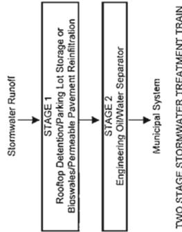
For major storm events where the attenuation and infiltration rates are exceeded, peak flows are directed to an engineered oil/water separator such as Vortechics or Stormceptor units. These engineered structures provide for greater than 80% removal efficiency for sediment and oil.
