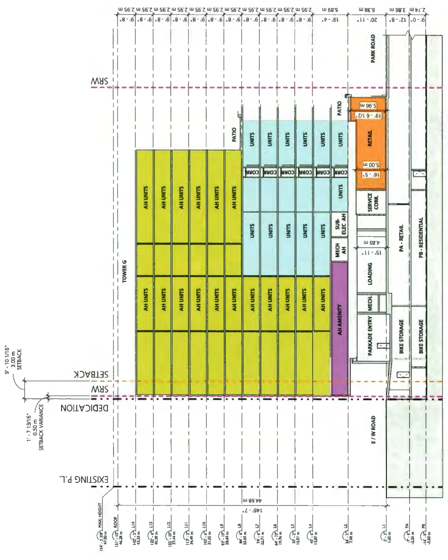
NORTH-SOUTH SECTION THROUGH TOWER G AT PARKADE ENTRY 1/16" = 1'-0"
