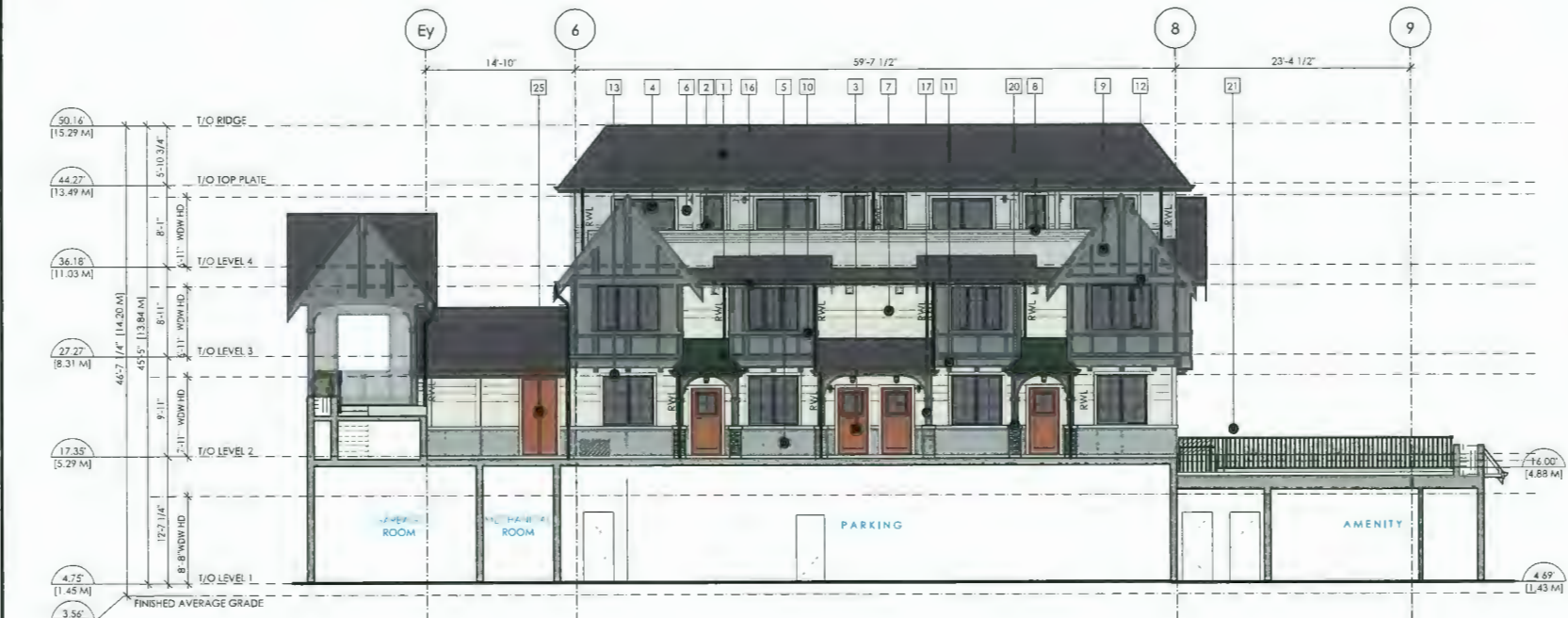
SOUTH ELEVATION BUILDING 2
