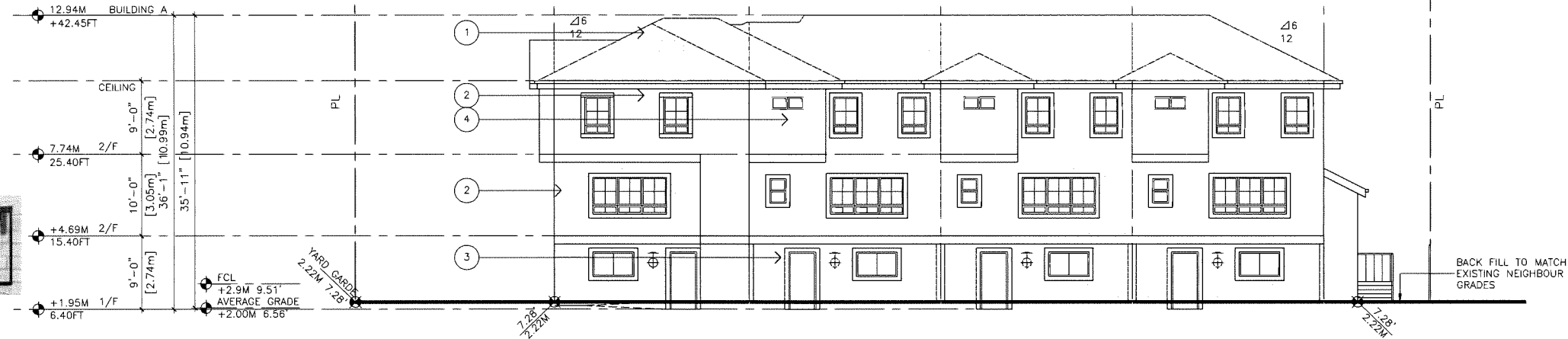
2 BLDG A WEST ELEVATION A9 1/8" TO 1'-0"
