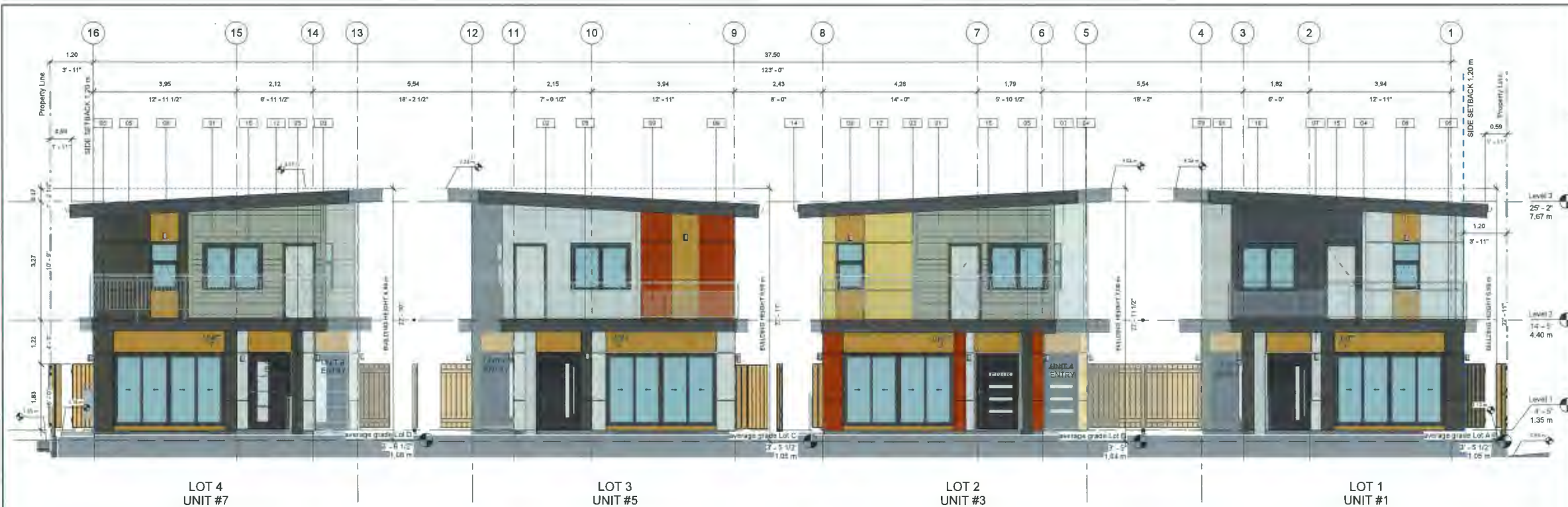
1 North (Front) Elevation 1/4" = 1'-0"
