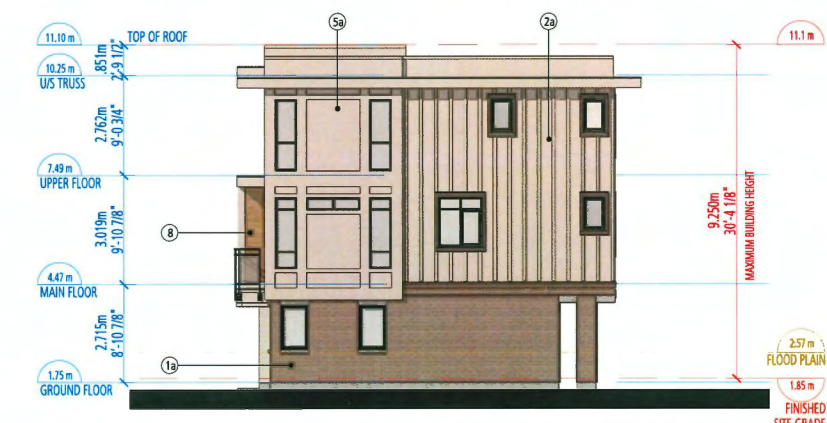
BUILDING 22 SOUTH ELEVATION
