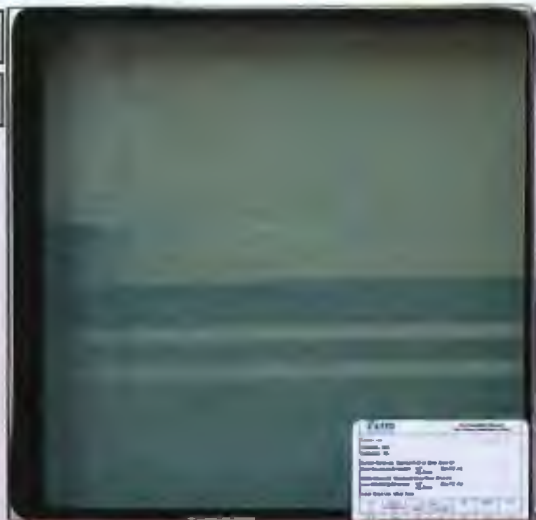
Solar Control Low-E Triple Insulated Glazing Unit Solarban 60*8mm + Air 12.7mm + Clear 6mm + Air 12.7mm + Solarban 60*8mm
