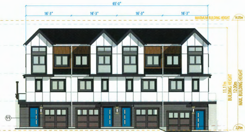
BUILDING 4 ELEVATION - SOUTH
