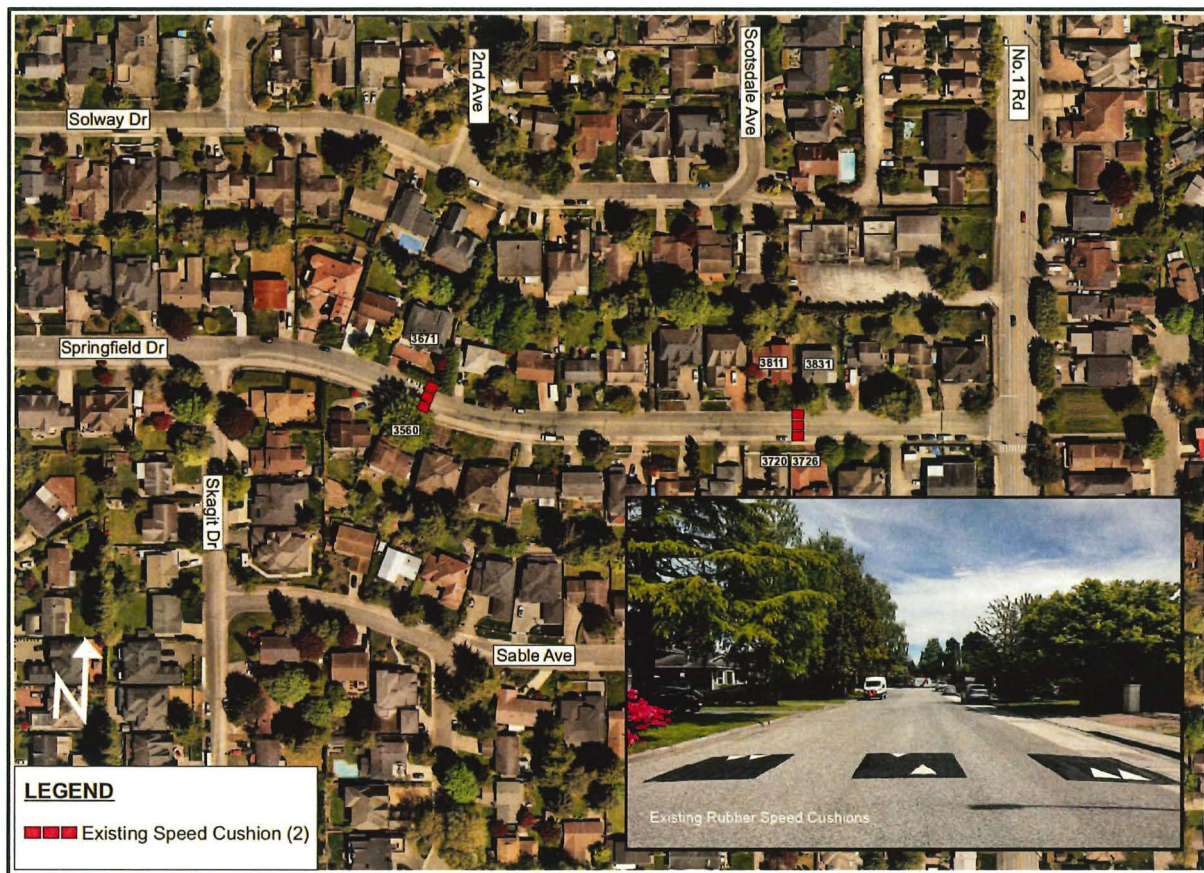
Figure 1: Springfield Drive Existing Rubber Speed Cushions
