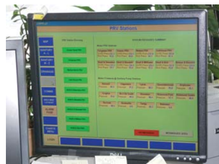
Pressure reducing valve (PRV) stations are monitored by S.C.A.D.A.
