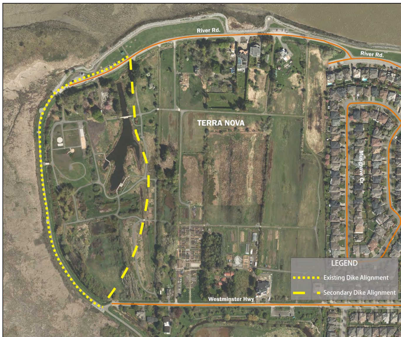
Figure 8: Secondary Dike Alignment through Terra Nova
