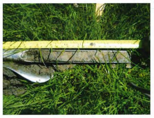
Figure 3 Soil sample showing mottled Bg horizon
