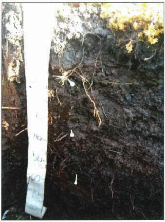
Typic Fibrisol. The watertable is at 33 cm in the pit.
