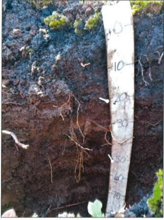
Typic Fibrisol, similar to the Triggs soil series.
