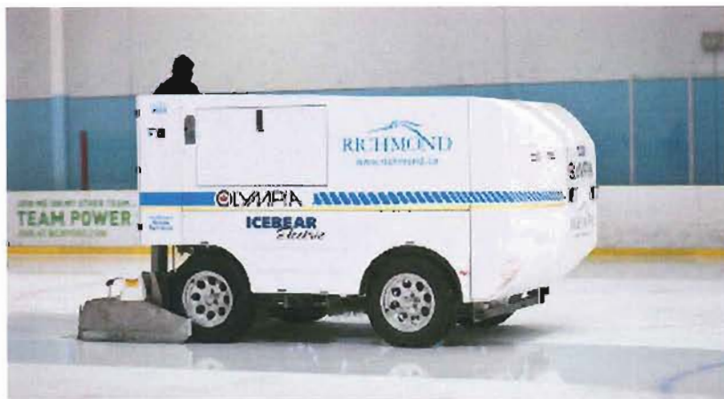
Figure 11. Richmond's ice arenas use electric ice resurfacers, eliminating fossil fuel use and improving indoor air quality
