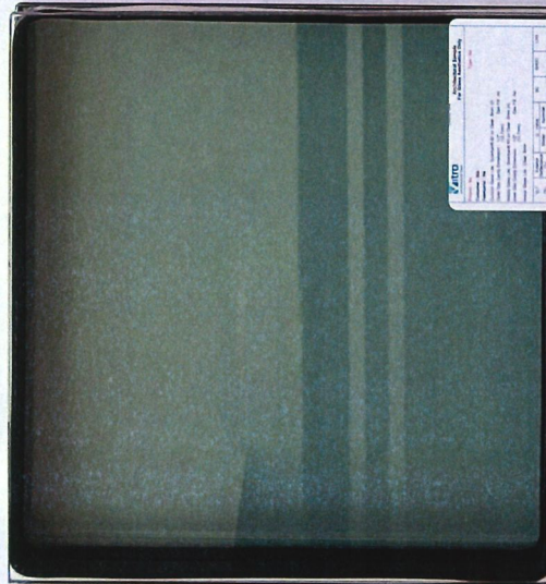
Solar Control Low-E Triple Insulated Glazing Unit Solarban 60'8mm + Air 12.7mm + Clear 6mm + Solarban 60'6mm
