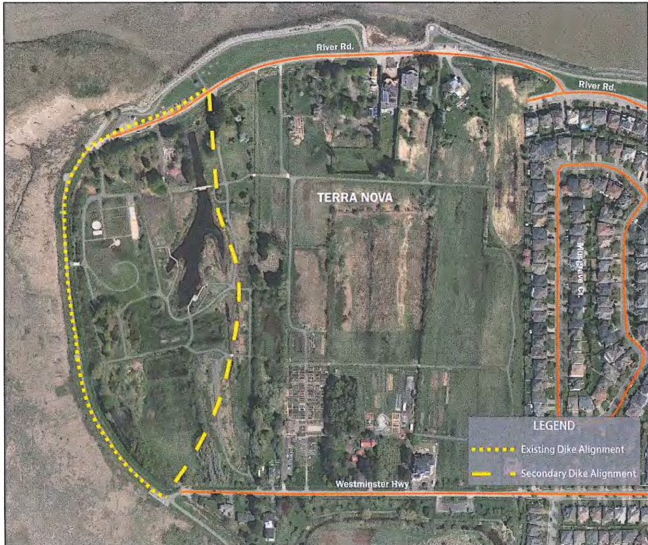
Figure 8: Secondary Dike Alignment through Terra Nova
