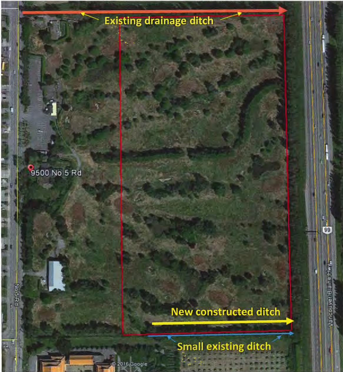
Figure 10 Location of surface drainage features
