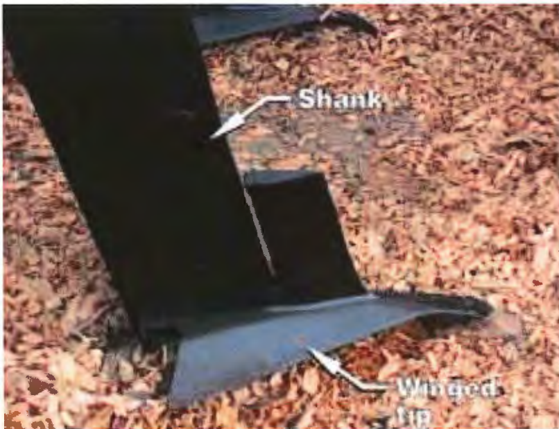
Figure 11 Example of a winged tine subsoiler
