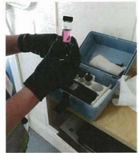
Testing the chlorine residual at the PVR
