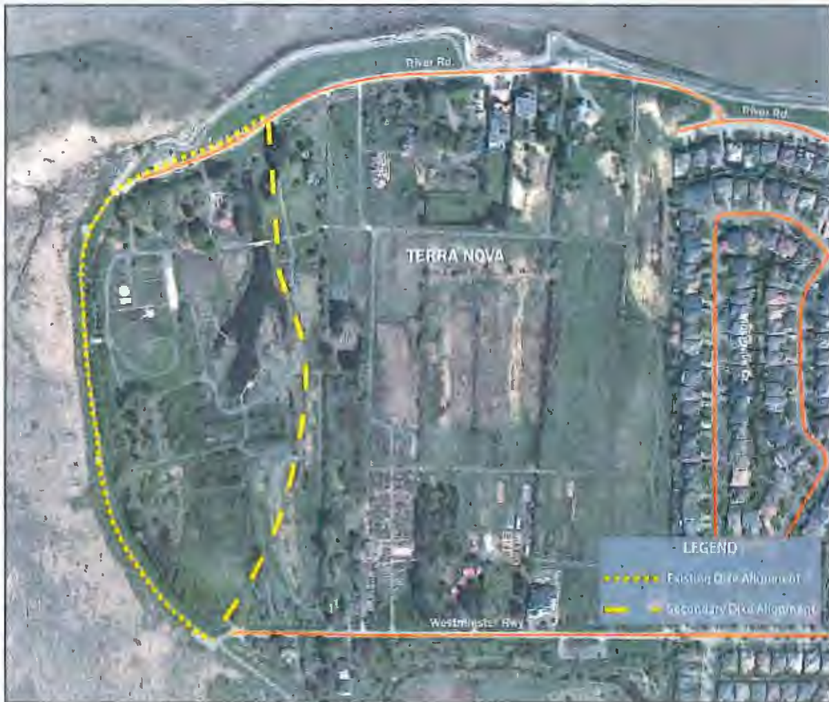
Figure 8: Secondary Dike Alignment through Terra Nova
