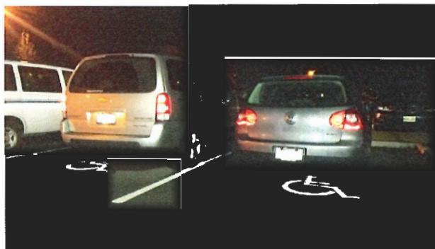
Figure 1: Side-Loading Van Unable to Deploy Ramp (photograph taken in jurisdiction outside Richmond)
