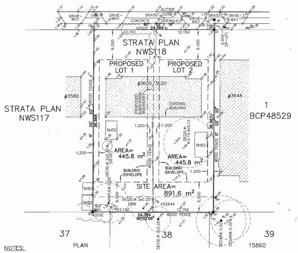
ELEVATIONS ARE IN METRES AND ARE DERIVED FROM CITY OF RICHMOND HPN MONUMENT #234 (77H4891) WITH AN ELEVATION OF 1.125 METRES.
