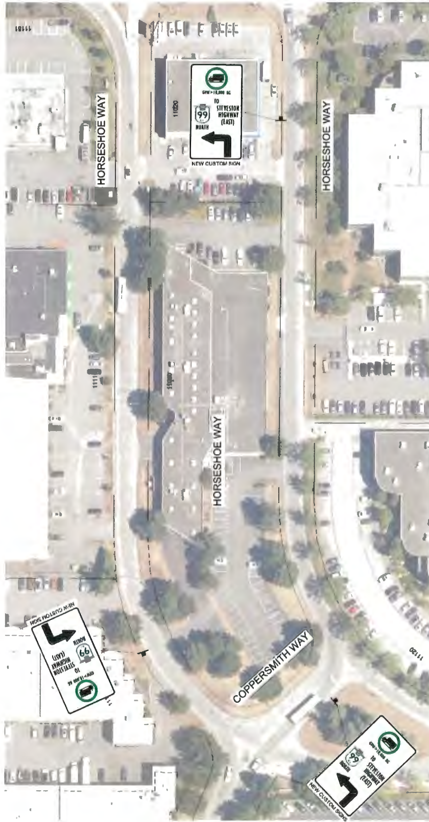
Shoulder-Mounted Signage for Truck Detour for Southbound No. 5 Road to Eastbound Steveston Hwy Left-turn Movement
