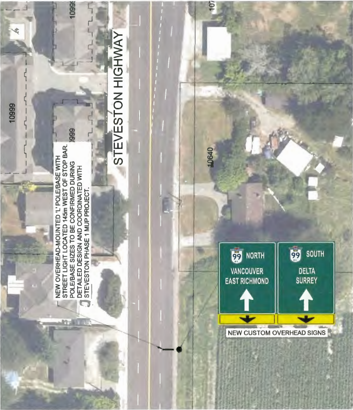
Overhead Signage on Steveston Highway west of Shell Road
