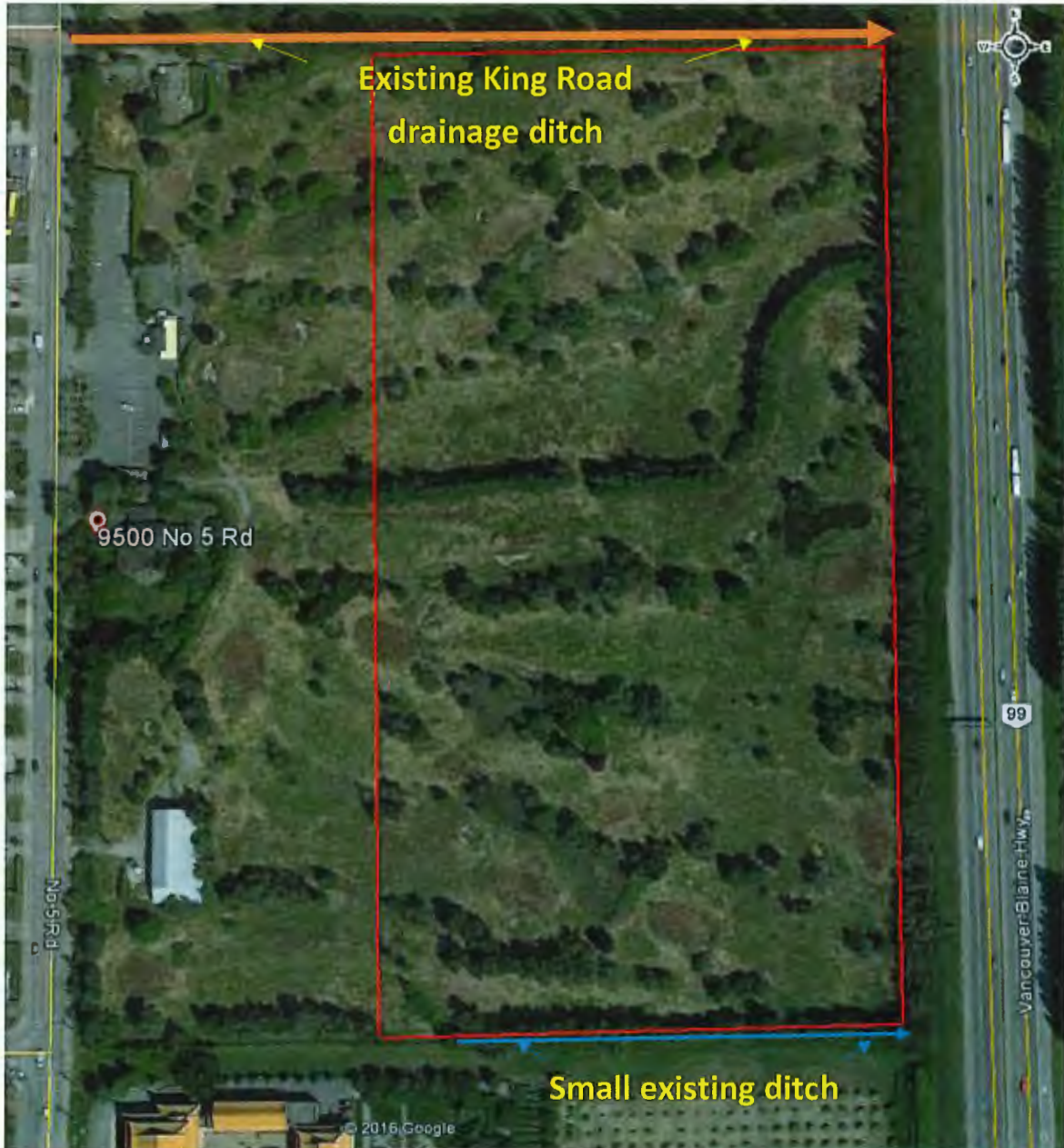
Figure 10 Location of surface drainage features
