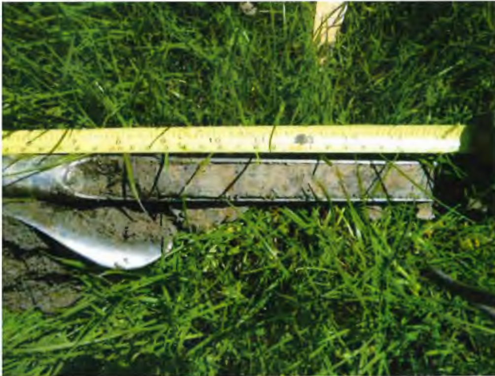
Figure 3 Soil sample showing mottled Bg horizon
