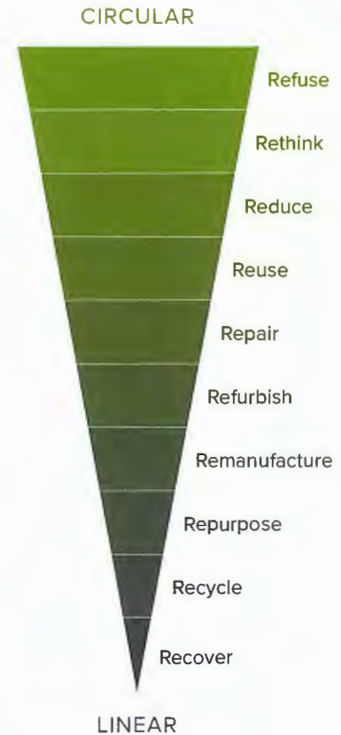
Figure 1: Circularity Ladder. We propose a circularity ladder, so called R-ladder. A variety of R-models are used to extend circular strategies, ranked in priority order. The R-ladder can be seen as a hierarchy where the highest possible step would be more ideal for a circular strategy.
