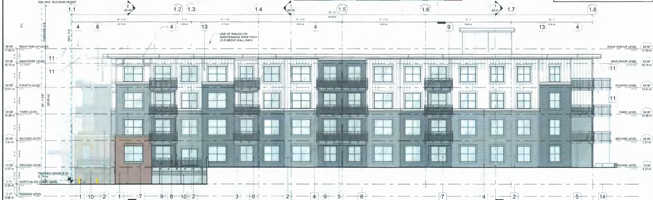
2 NORTH BUILDING - WEST ELEVATION A4.00 1/8" = 1'-0"
