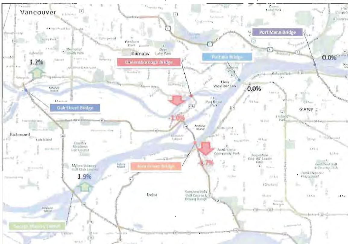
Figure 4. Difference in Truck trips 8-lane bridge (tolled) vs. 4-lane tunnel (untolled) – 2045 AM Peak Hr
