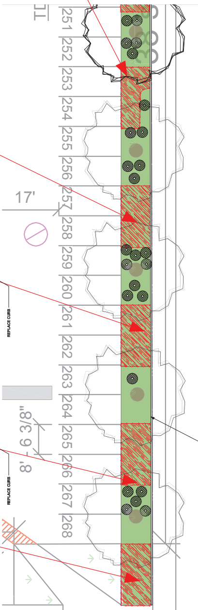
2 Landscape Demolition and Retained Plant Plan West Scale: 1/8" = 1'-0"
